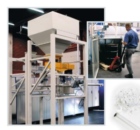
The Continuous Flow Distiller from MRT System is the result of continued development and adaptation to requirements from the waste management companies and the lamp industry. The distiller version being a solution especially designed for high capacity requirements, manages treatment of up to 5 times larger quantities of fluorescent powder and other low organic materials compared to a standard distiller.
