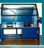
The manually operated system is a simple version, it can process CRTs ranging from 8" to 40". The operator measures, scratches and applies the hot band manually.
