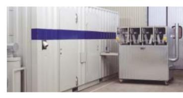
To eliminate the risk of mercury and dust particles being released during the process, the entire system works at sub-pressure. A high capacity fan incorporated in the system represses all hazardous mercury vapours and allows the operator to work in a dust free environment.
