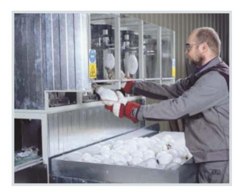
The MRT HID Processor is designed for safe processing of High Intensity Discharge (HID) lamps of various types and sizes. This equipment not only reduces the volume of discarded lamps, but ensures reliable disassembly and isolation of the mercury bearing components.
