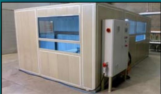
The FPP is enclosed in a ventilated compartment. The ventilation package is a powerful system incorporating blower, dust separator and carbon filters which ensure a safe and reliable recycling process.
