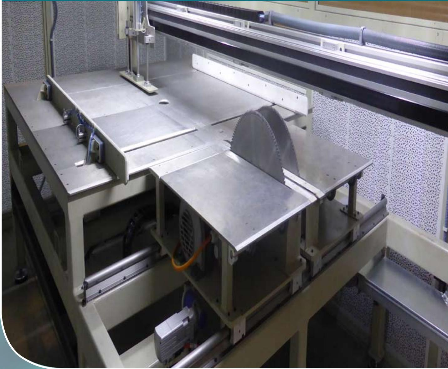
**The flat panel processor (FPP60)** is a versatile machine designed to disassemble a large range of flat panels. The processor allows for secure extraction of the fluorescent lamps and separation into the different fractions.
